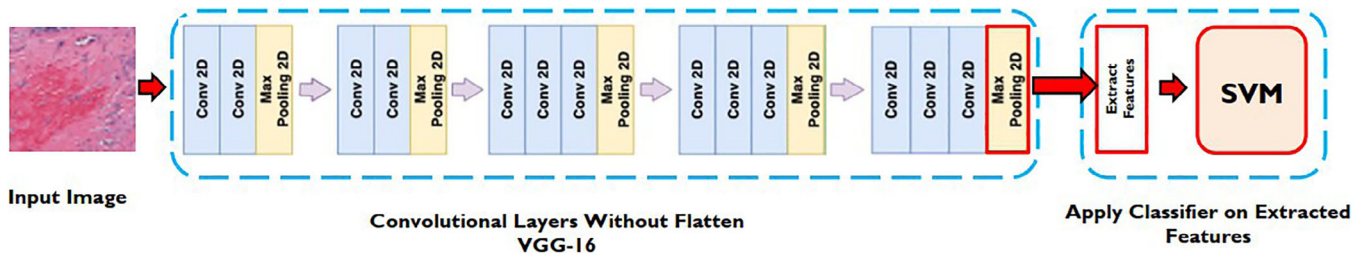
FIGURE 4 | The architecture for the suggested approach to the detection of breast cancer.
